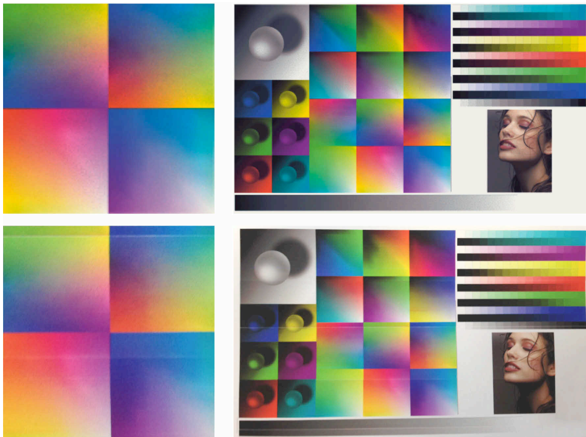
Figure 4: Simulated print (top) and photo of print (bottom) derived from the same halftone data.
