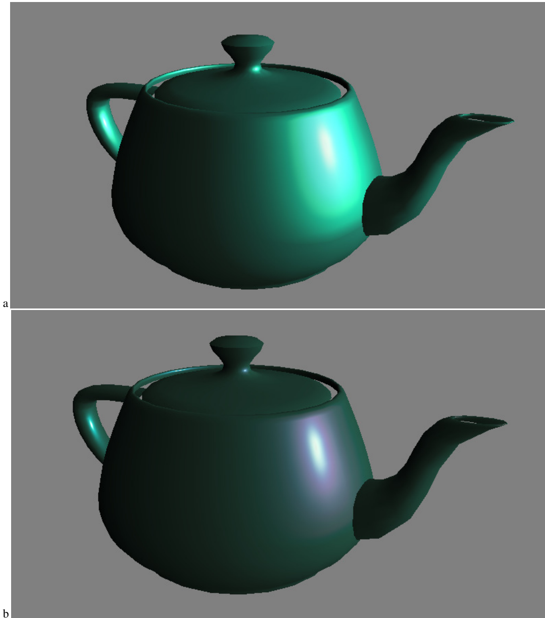
Figure 7. In these 3D rendering examples of the Utah teapot we used the isoline-based rendering method developed in this article, using the proposed clipping method. Color information is based on the BRDF measurements on metallic sample 7 from Ref.[12], and extreme interference sample 13.
