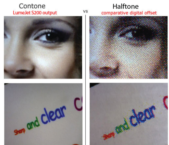
Fig.4 LumeJet contone quality compared to halftone digital offset.
