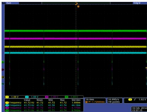
Figure 6 – Phase-frequency synchronicity of four frames.
