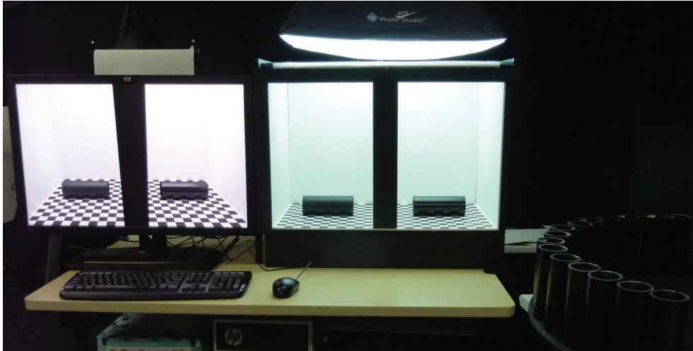
Figure 1. Setup used for the experiment. From left to right, 30-inch HP ZR30w display, custom-built light booth, and lazy susan used to provide easy access to the samples to the users. The color difference seen between the different media is due to the camera response.
