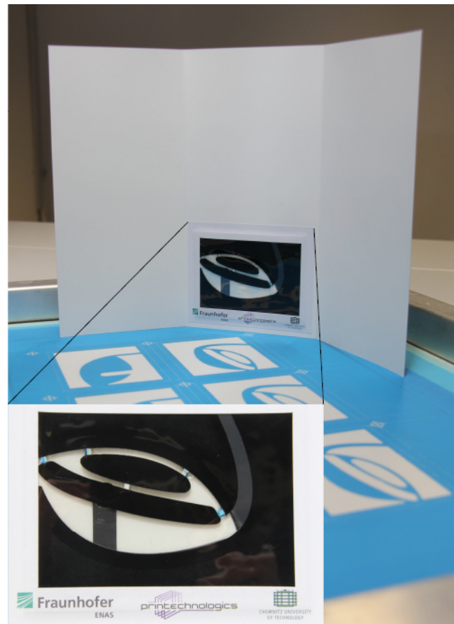
Figure 4. Integration of the smart system to a card demonstrator; including a zinc-manganese battery, a push-button and assembled components
