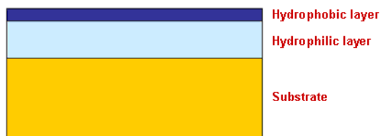
Figure 4. The samples used in the experiments consist of a polymer substrate with a hydrophilic and a hydrophobic coating on top of it.
