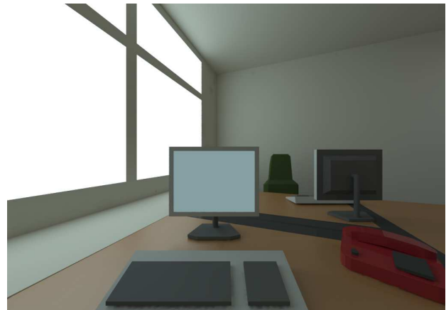
Figure 3. Office test scene: view from the front workplace. This view is important for the evaluation of the circadian action factor a_{cv} as it simulates the field of view of a person working at the desk.
