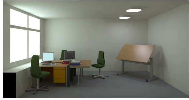
Figure 2. Office test scene: overview. The test scene contains three different sources of illumination: four light sources that simulate the windows, two LED ceiling lamps, and two computer monitors.
