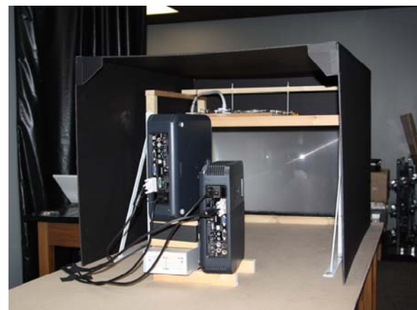
Figure 3. High dynamic range display: (top) front view showing LCD panel, (bottom) rear view showing tiled DLP projectors.
