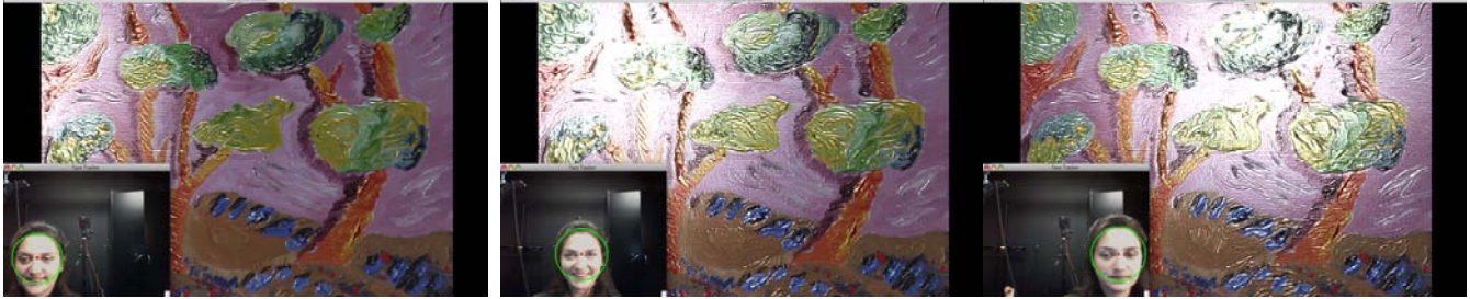
Figure 4: Dynamic viewing: The three screenshots illustrate the dynamic viewpoint control capabilities of the tangiBook. The insets show the output of the webcam-based headtracking software as the observer moves from left to right. The large images show the corresponding movement of surface reflections.
