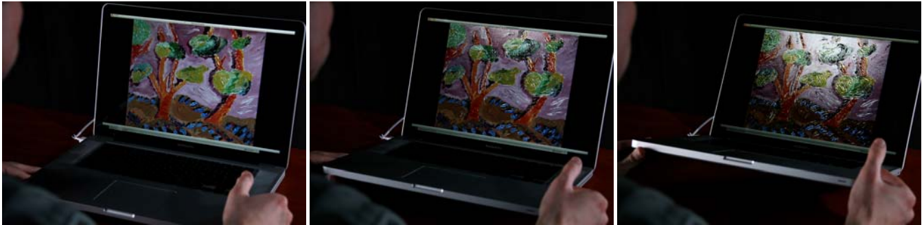
Figure 1: Image sequence showing a painting model being displayed on the tangiBook. The tangiBook is based on an off-the-shelf laptop computer that incorporates an accelerometer and a webcam as standard equipment. Custom software allows the orientation of the laptop screen and the position of the observer to be tracked in real-time. Tilting the laptop (as shown) or moving in front of the screen produces realistic changes in surface lighting and material appearance.
