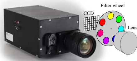
Figure 1. Seven channel multispectral camera with its internal configuration sketched.
