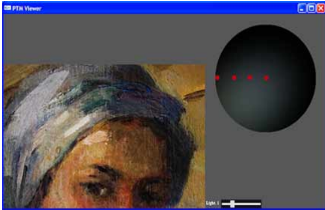
Figure 6. The PTM Viewer showing the selected locations of the light sources. Painting by Michèle Stapley
